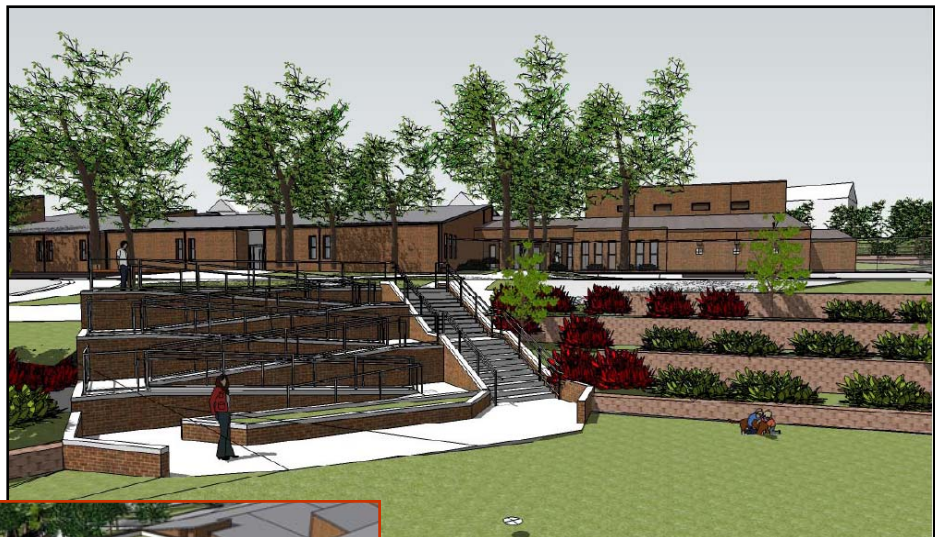
A three-tiered micro-bioretenion area and a green roof are part of the addition of a new gymnasium at Cold Spring Elementary School in Montgomery County.
